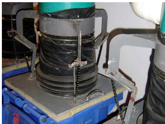
Figure 4 Air tight bin cover
