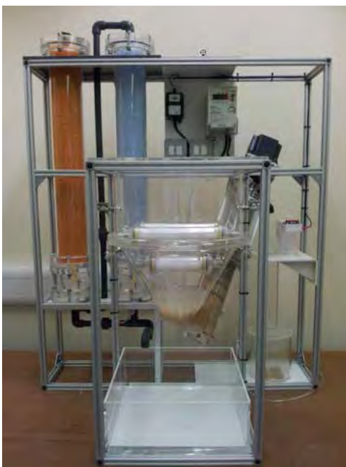
The works-like prototype processing synthetic urine and feces.
