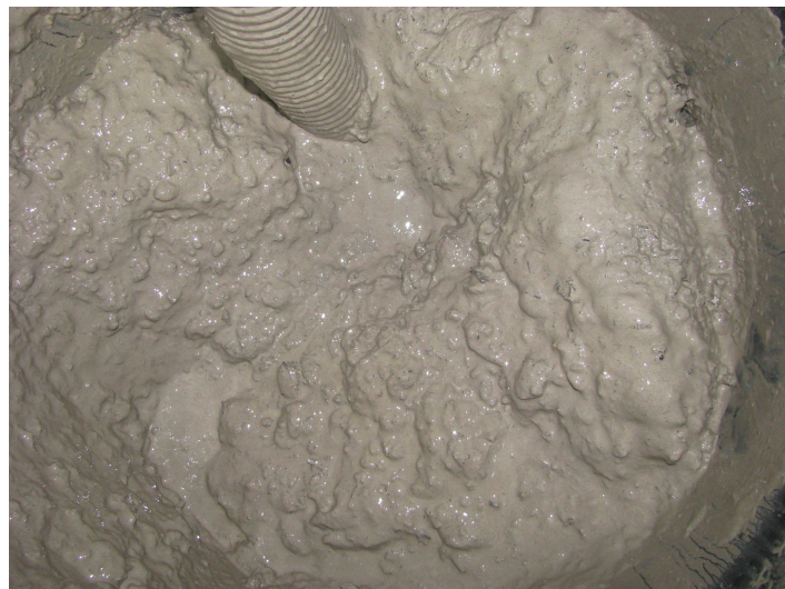
Figure 17: Residual sludge in tank after fluidisation and emptying
