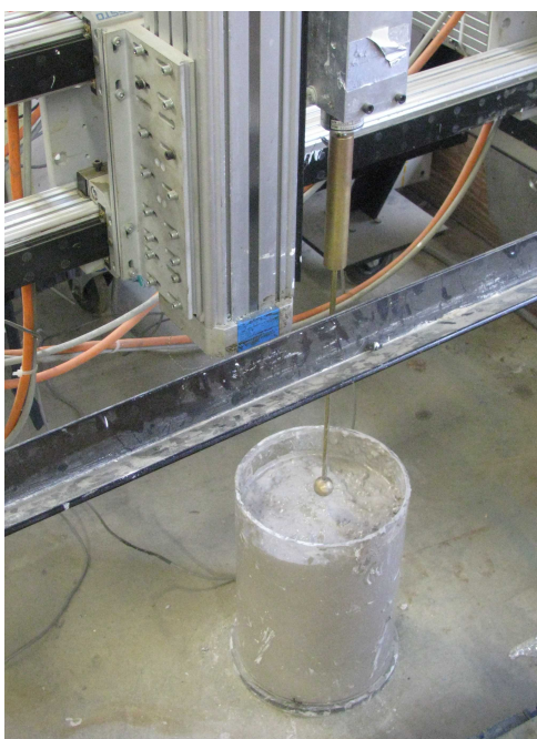
Figure 2 (a): Mini-ball penetrometer in testing rig
