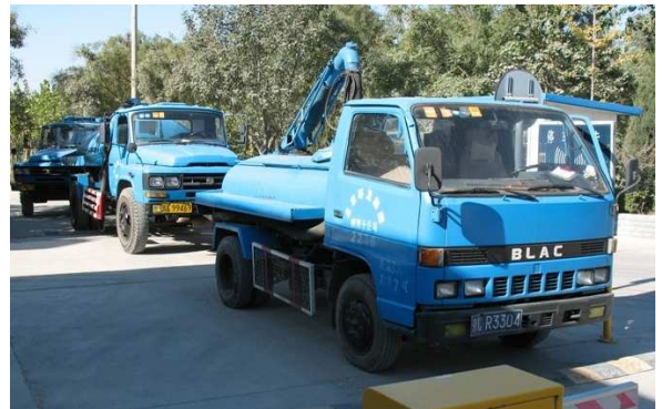
Fig. 7: Type of vacuum trucks to be used for the transport of scum and sludge from the septic tanks at the public toilet blocks with low flush, urine diverting toilets in the Olympic Forest Park. This picture was taken at an MBR wastewater treatment in metropolitan Beijing.
