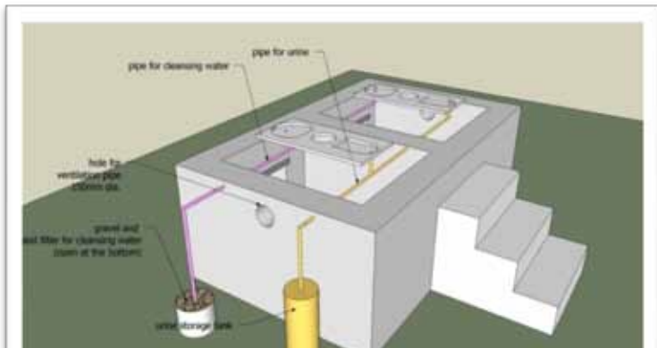
Figure 17: Schematic Arrangement of Urine and Anal Cleansing water Pipe and Collection Tanks
