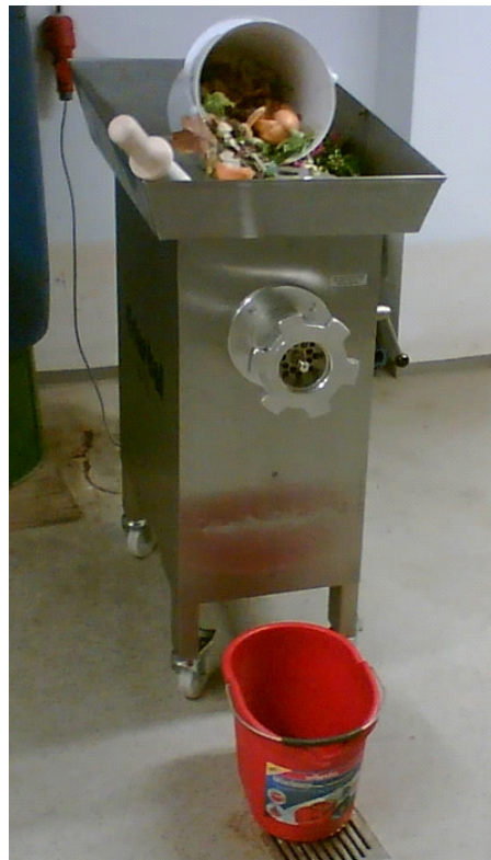
Fig. 2.4.22: Grinder (Edertal 2007) for bio-waste for biogas plant
