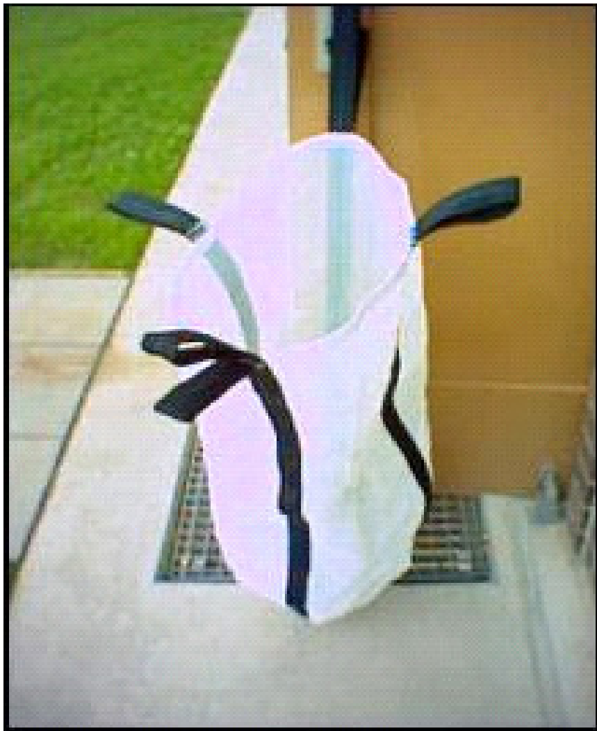
Fig. 2.4.9: Fugafil-Saran Filter bag (PE 1200/500) for faeces dewatering
