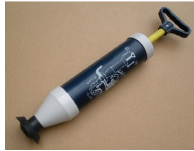
Fig 4: Manual suction pump for the cleaning of urine pipes
