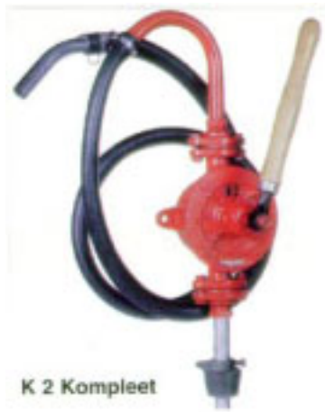
Photo 7.3 Example of hand pump (semi-rotary pump) suitable for this situation: small and light with a suction depth of more than 5 meters and an acceptable capacity of 25-50 litre/minute (depending on the type of the pump and strength of operator)
