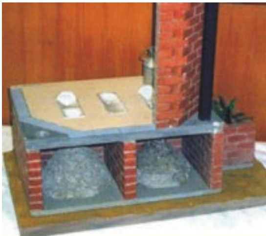
Photo 8.4 Dried collection of faeces: use of double vault system and the result Left picture: The two chambers under the toilet slab where the faeces are collected and are dried with time. (Photo: Agricultural University of Norway) Right picture: The result: the dried faeces taken out of a double vault system
