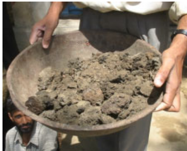
Photo 8.4 Dried collection of faeces: use of double vault system and the result Left picture: The two chambers under the toilet slab where the faeces are collected and are dried with time. (Photo: Agricultural University of Norway) Right picture: The result: the dried faeces taken out of a double vault system
