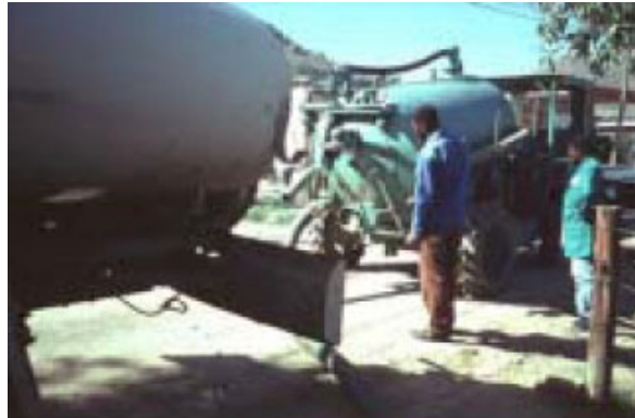
Photo 8.3 Wet collection of faeces: an example of a mini vacuum tanker and transfer Left photo: a 500 litre mini tanker (pedestrian controlled and in traction mode, the engine can propel the vehicle at speeds of up to 5kph) (Source picture: UN-HABITAT, 2005) Right photo: Transferring the faecal sludge from a small sized tanker to a large sized tanker (Source picture: Strauss)
