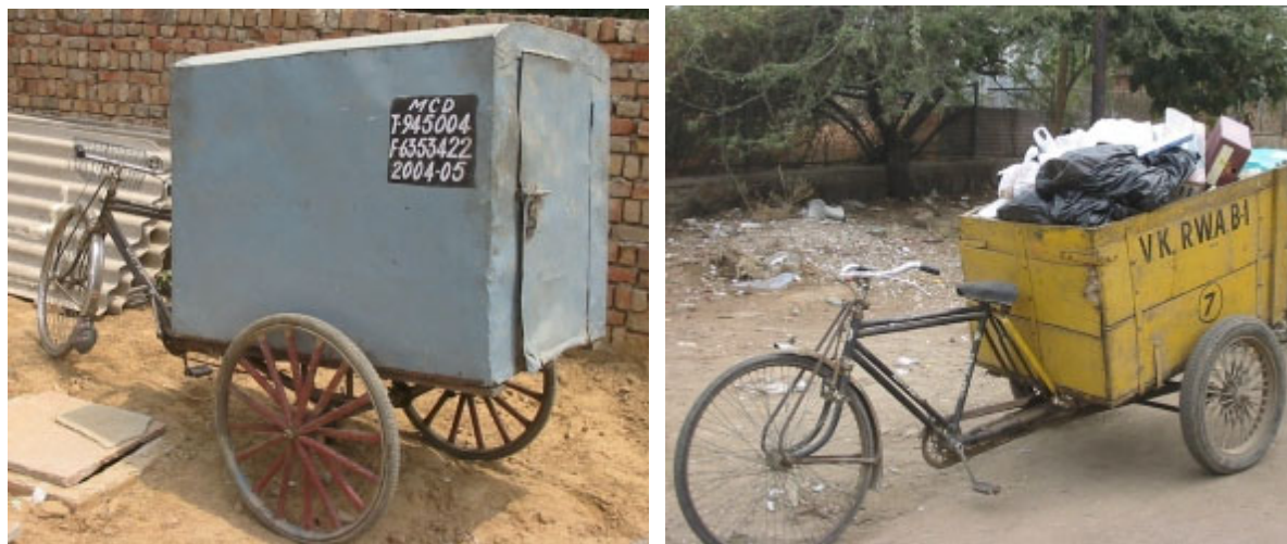
Photo 8.5 A closed body tricycle and and the heightened sides of a tricycle body (photos related to text on next page)
