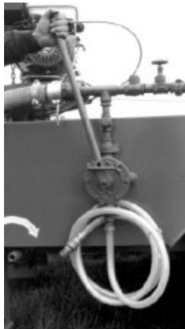
Photo 7.3 Example of hand pump (semi-rotary pump) suitable for this situation: small and light with a suction depth of more than 5 meters and an acceptable capacity of 25-50 litre/minute (depending on the type of the pump and strength of operator)
