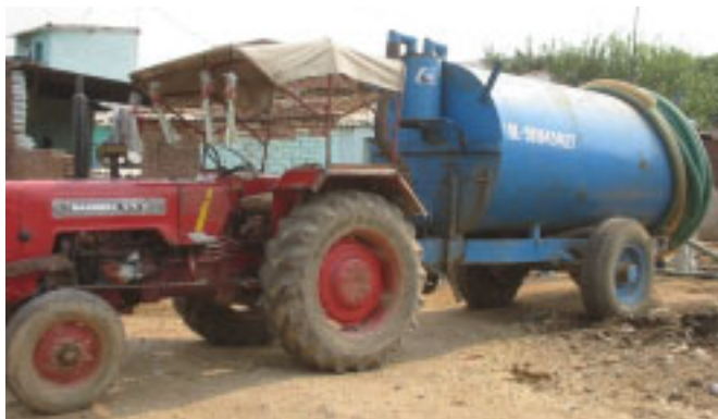
Photo 8.2 Wet collection of faeces: use of vacuum tankers These can be made in different sizes (Right picture: Esrey, 1998)
