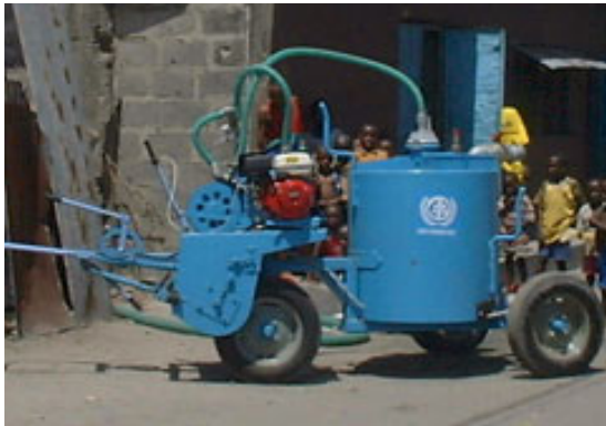
Photo 8.3 Wet collection of faeces: an example of a mini vacuum tanker and transfer Left photo: a 500 litre mini tanker (pedestrian controlled and in traction mode, the engine can propel the vehicle at speeds of up to 5kph) (Source picture: UN-HABITAT, 2005) Right photo: Transferring the faecal sludge from a small sized tanker to a large sized tanker (Source picture: Strauss)
