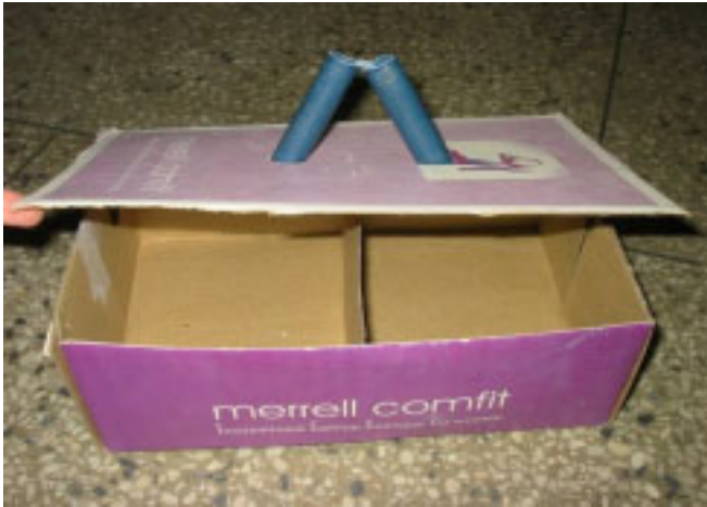
Construction representing basic double vault chambers and a urine-diverting toilet
