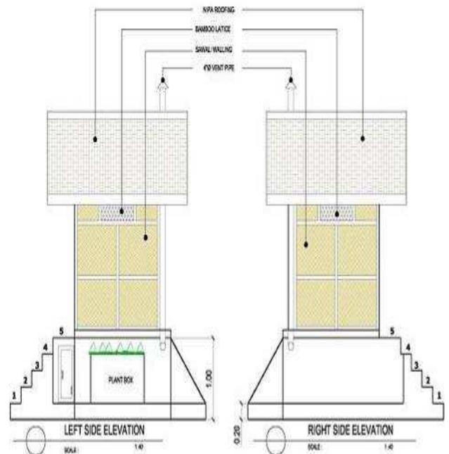
**Fig. 6:** Design drawings for double-vault UDD toilets – Part 2 of 2 (design drawings provided by Dr. Holmer from PuVep, see <http://puvep.xu.edu.ph>)
