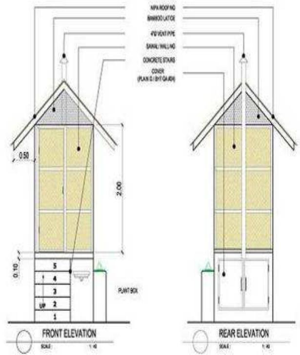
**Fig. 5:** Design drawings for double-vault UDD toilets – Part 1 of 2 (design drawings provided by Dr. Holmer from PuVep, see <http://puvep.xu.edu.ph>)
