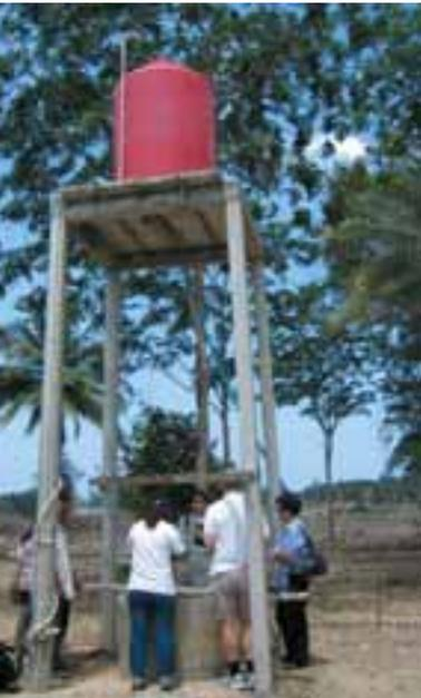
Surveying in the tsunami zone. Water level was measured in every well and related to sea level.
