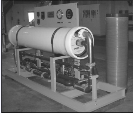
Figure 17: MegaMagnum® RO Element (picture by Harm Jansen)
