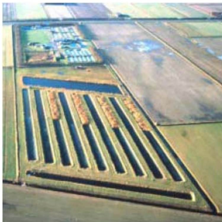
Figure 3.44: Eversteekoog: Aerial View of the Eversteekoog constructed wetland, on the background the STP (photo Simon Smit, Texel)
