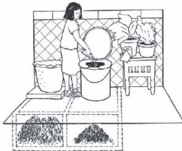
Figure 17: Double-vault urine-diverting dry ecosan toilet [60]
