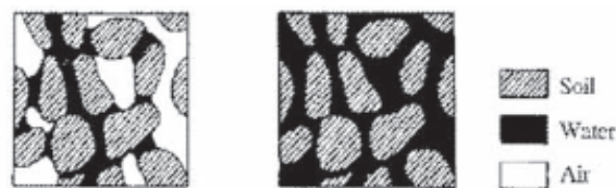
Figure 43: Unsaturated flow (left) gives better filtration and oxygenation of the water than saturated flow (right) [59]
