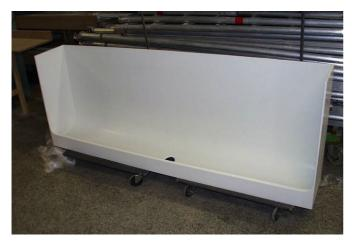
**Fig. 6:** A urinal trough (2 m width) before installation, made of marble powder (source: P. Grönwall, 2006). The outlet in the middle has a Keramag flat rubber tube for odour control, see photo below.
