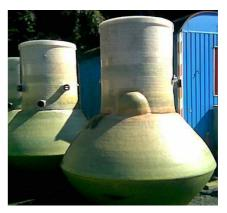
**Fig. 5:** Glassfibre reinforced plastic (GFP) tanks for urine storage before installation (volume 2.5 m3). These tanks are buried next to the urinal shed (source: P. Grönwall, 2003).
