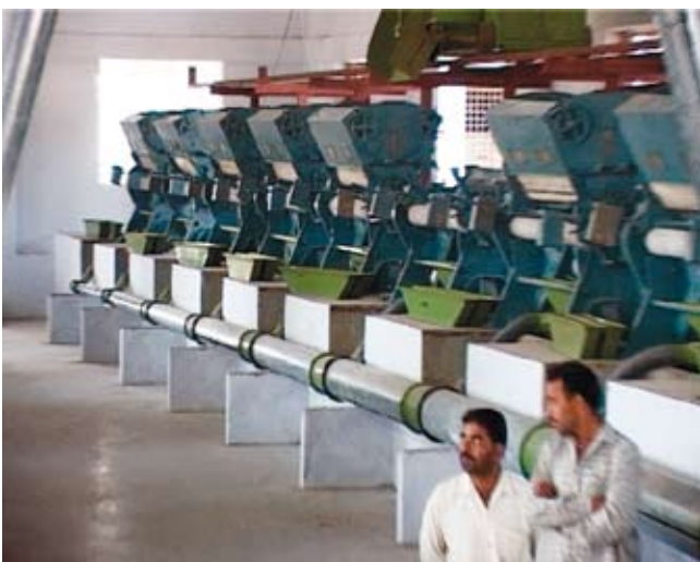
The first processing step for cotton is the ginning factory where the seeds are extracted and cotton lint is produced
