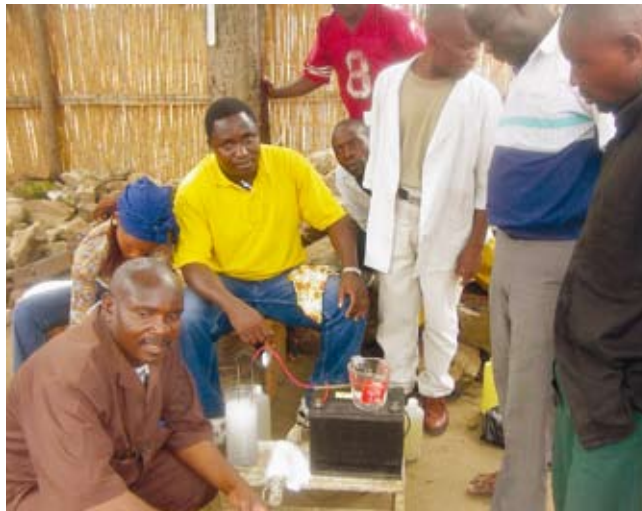
Antenna's small chlorine factory allows for decentralised production with simple means: electricity and cooking salt
