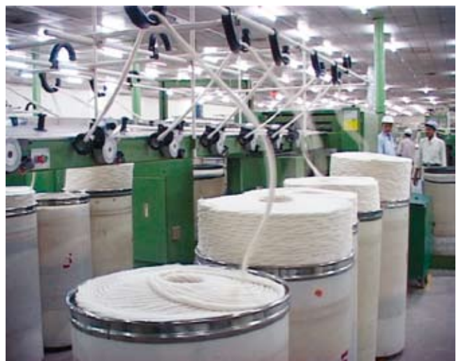
The next step is spinning of yarn. One kg of cotton lint produces 0.65 kg of cotton yarn.
