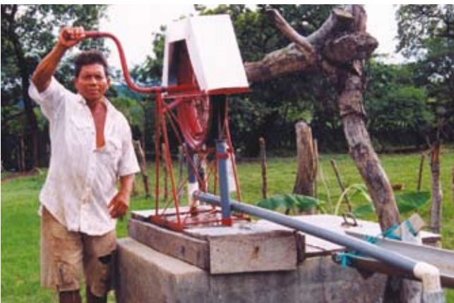
The rope pump, Central America
