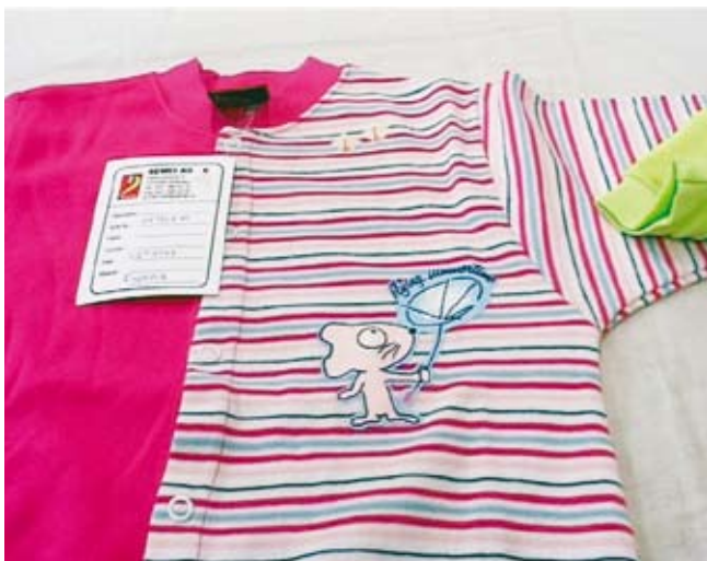
This baby pyjama has three colours that need to match: the left side is dyed cloth, the stripes are dyed yarn and the figure is printed
