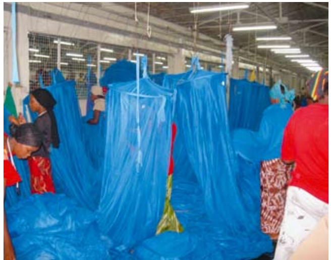
A to Z is a large textile mill in Arusha now producing long-lasting nets; the insecticide is already dissolved into the polyethylene granules
