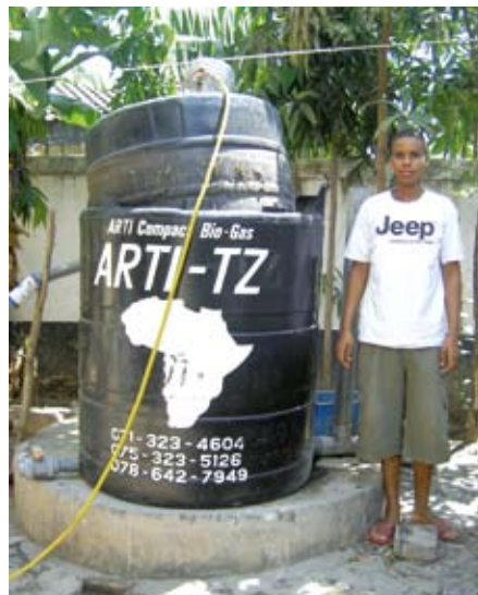
Photo 1: ARTI household digester in Dar es Salaam, Tanzania.
