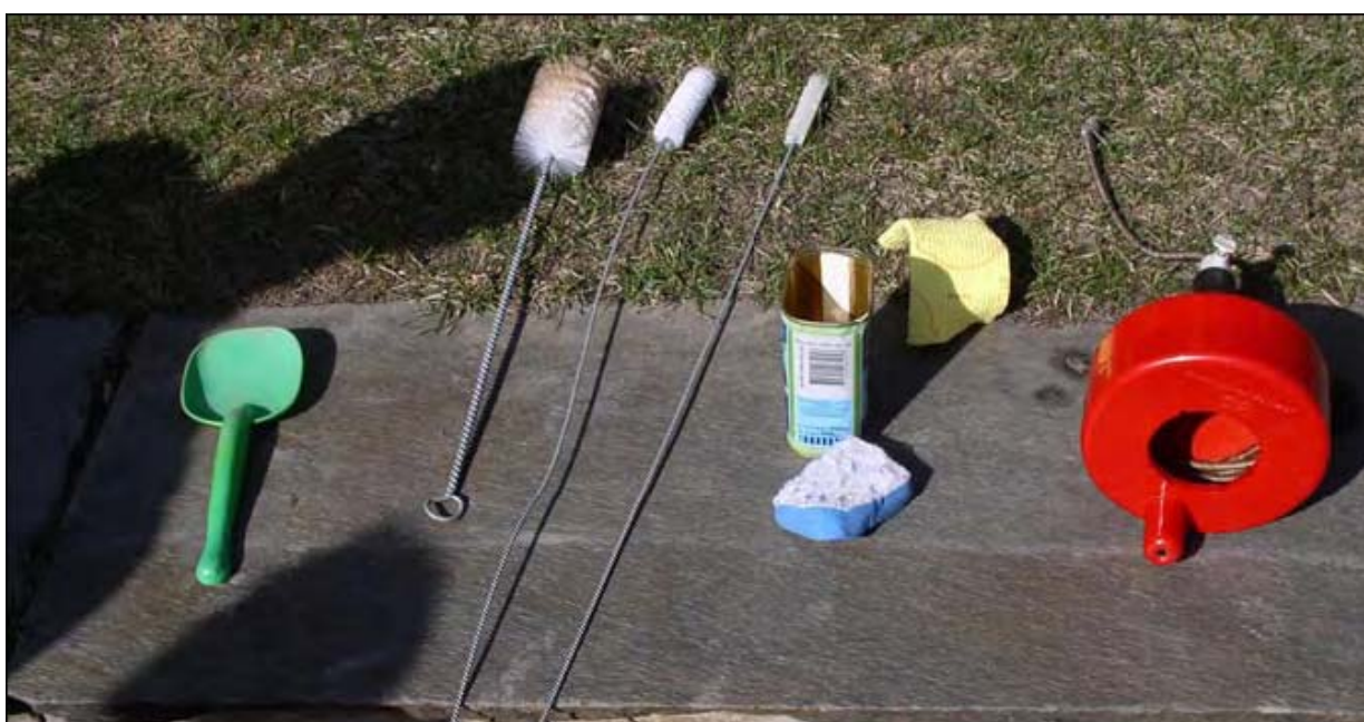
Figure 5: Cleansing tools for urine pipes [8]
