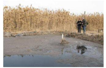
**Fig. 10:** Foreground: primary sludge drying bed (was: reed bed for primary sludge conversion to soil). Background: reed beds (source: E. v. Münch, Jan. 2009)
