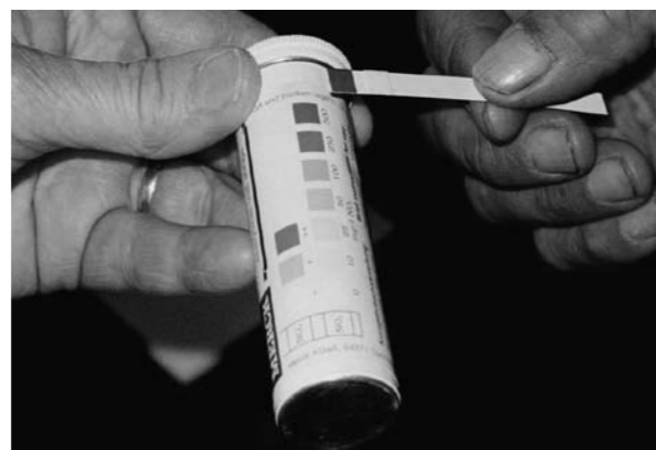
Example of a nitrate quick-test: this particular test showed that the drinking water well had a very high level of nitrate.
