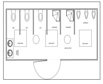
Figure 5: Typical design of a CAB (source: EWS, 2009).
