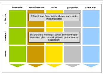
**Figure 2:** Applied sanitation components in this project (currently no reuse taking place).
