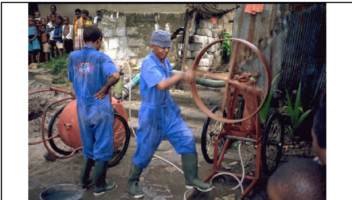
Figure 1: The MAPET, developed by the Dutch NGO WASTE, in action in Dar es Salaam (photograph by Jaap Rijnsburger)
