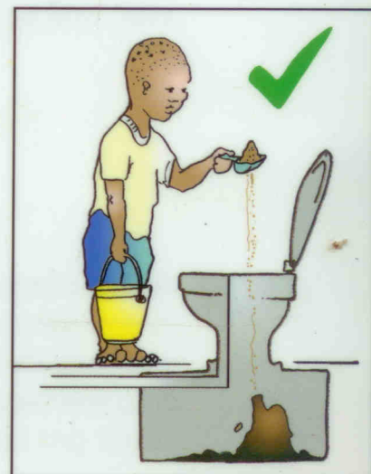
3. Ash or sand is thrown over faeces after each use. Do not pour water into the pit.
