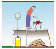
Do not pour water with chemicals into the vault for cleaning.
