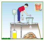
Ash or ash with soil is thrown over feces after each use. Do not pour water to the pit.
