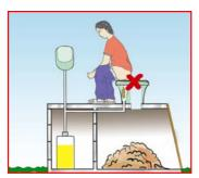
Do not defecate into the front (urine chamber) of the toilet.
