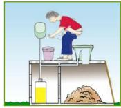
Throw anal cleansing materials into a separate container next to the toilet. They should be burned or buried.
