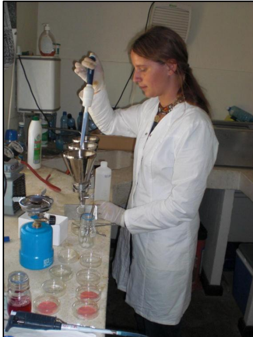
Figure 12: Membrane filtration for faecal coliforms
