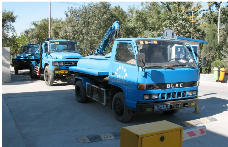
Pic. 2: Vacuum trucks delivering waste water to a MBR waste water treatment plant in Beijing
