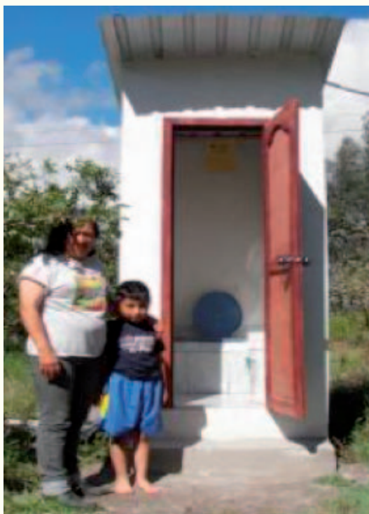
Figure 5: Finished UDDT in use. Mrs. Mélida T. is one of the most enthusiastic users. She and her family of four filled 2.5 sacks in six months, fertilize vegetables and fruit trees with the urine, and look forward to using the soil conditioner. (Photo: C. Canaday)
