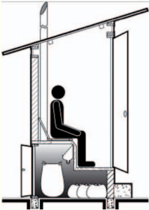
Figure 1: UDDT Design. Interior dimensions were 120 cm long by 90 cm wide
