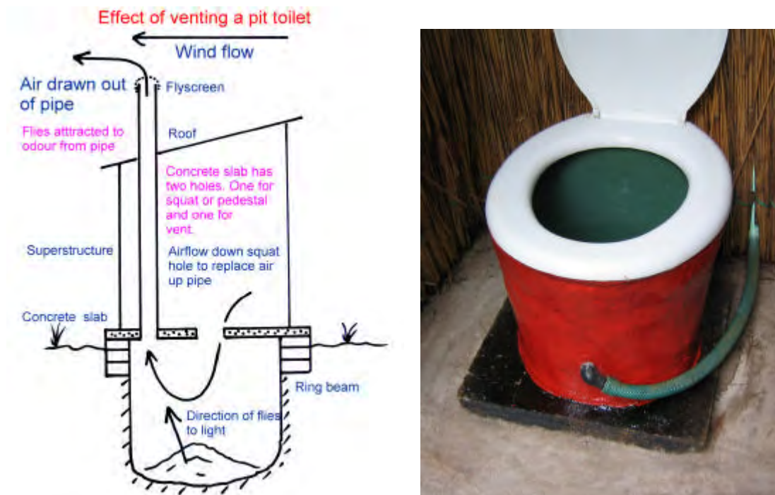
Left: Diagram showing effect of vent pipe on controlling odours and flies. Right: A urine diverting pedestal with above slab urine take-off. This type is suitable for upgrading shallow pit composting toilets like the Fossa alterna to urine diversion. Pits under urine diverting pedestals are drier and this helps to control flies and odours.
