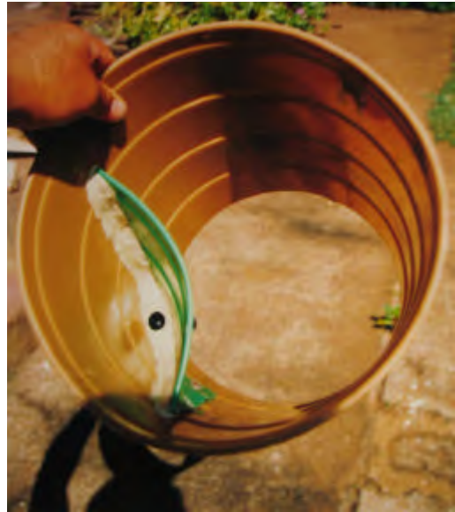
In this method a piece of plastic from a bucket is bolted to the side wall of the larger chute bucket to make the urine diverter. At the base of the diverter a polyethylene pipe is fitted in place with epoxy putty. Urine passes down the diverter, through the pipe into the urine storage vessel. This plastic unit is then built up in cement and a seat is fitted as described earlier.
