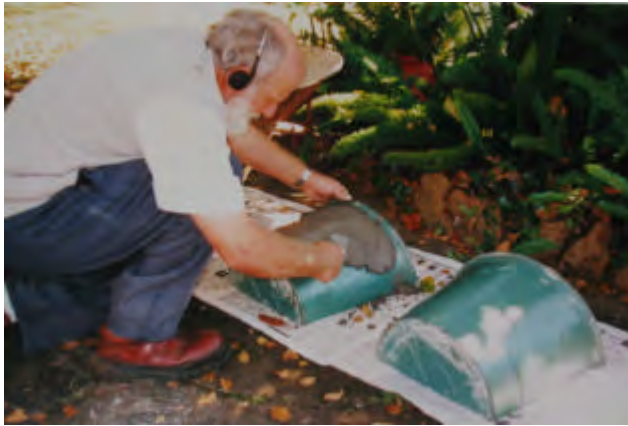
Plastering the two shells of the 30 litre split cement jar on a mould made from a 30 litre plastic bucket. After a few days of curing the two cement shells can be separated from the mould.
