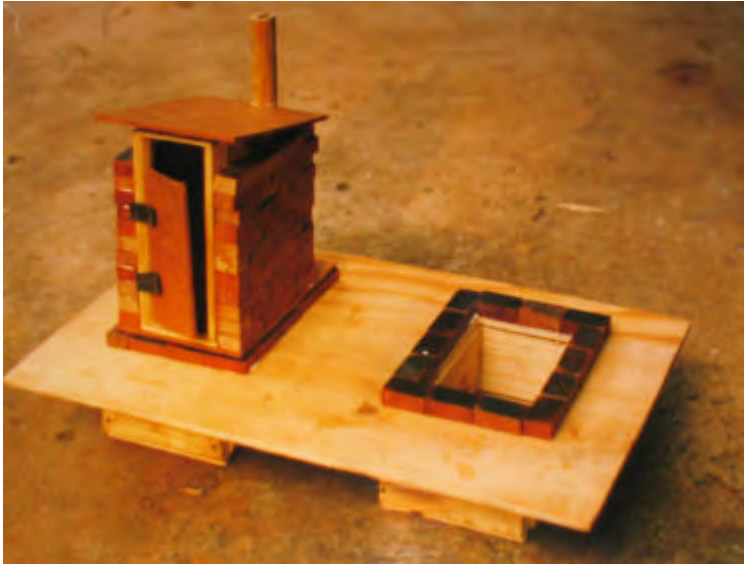
On the left a small wooden model of Fossa alterna . On the right a one third scale model of the Fossa alterna with concrete ring beams and slab, and wooden from a vent pipe.
