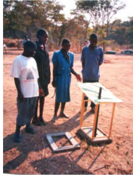
On the left a small wooden model of Fossa alterna . On the right a one third scale model of the Fossa alterna with concrete ring beams and slab, and wooden from a vent pipe.
