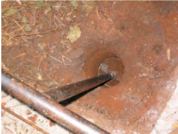
On the left samples of Fossa alterna soil are taken with an earth auger. The auger is drilled down to specific depths and samples withdrawn and placed in sample bottles. On the right the hole has been drilled down to 60cm (total soil depth was 64cms).
