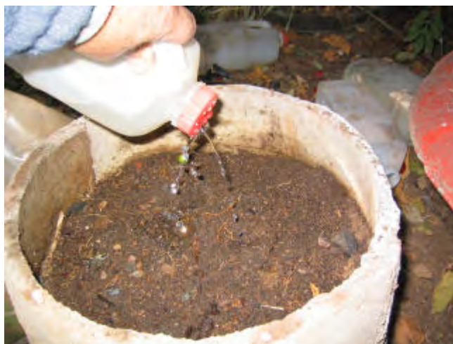
The “cocktail” was then added to a jar of composting soil and excreta taken from the Skyloo . After one month the soil was tested in the laboratory and none of the lethal bacteria could be found.
