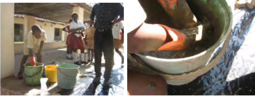
The cement and salty water are mixed in a large bucket and thoroughly stirred using rubber gloves.
