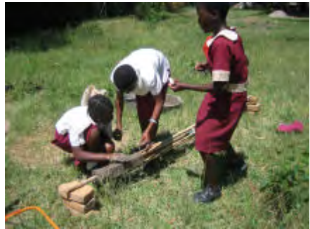
Full length pipes being covered with cement and sand impregnated cloth at Chisungu school. The technique takes a bit of practice to get it right.
