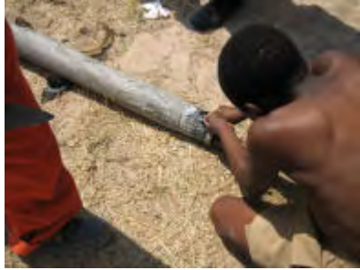
The pipe after curing. Removing the folded plastic sheet
