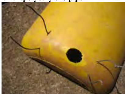
A hole is also cut with a sharp knife in the cut section of bucket at the lowest part where the urine will collect
