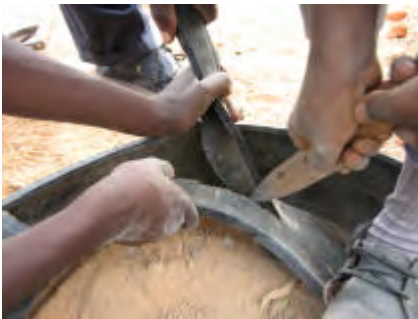
Pupils cutting the rubber hinges from car tyre.
