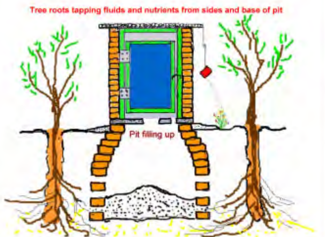
Diagrammatic view of root growth formation around porous pit lining
