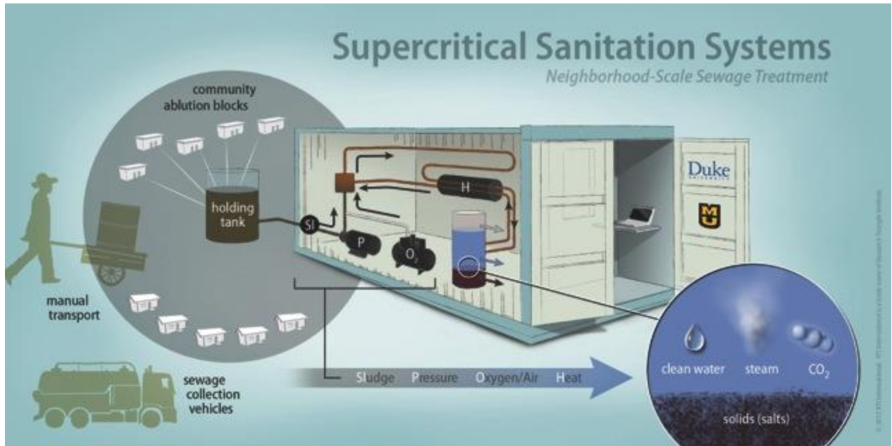
Figure #2: Illustration of the Duke-Missouri SCWO Technology. Source: Duke University (2013).
