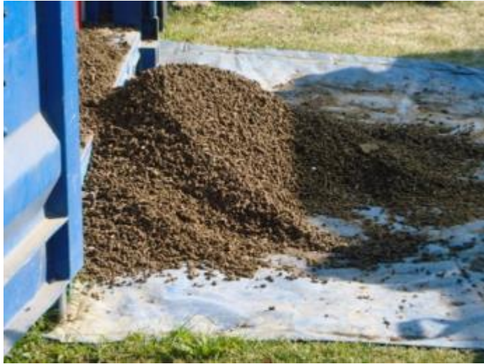
Photograph 5: LaDePa technology removes garbage from the solid waste, heats the waste and effectively removes all pathogens, and turns the waste into pellets used as fertilizer.
