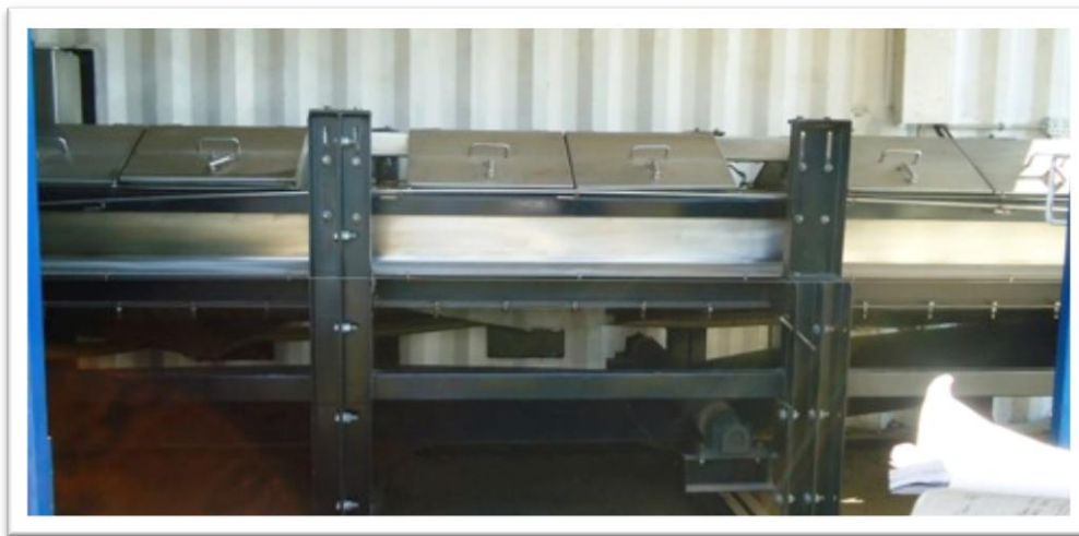
Figure #12: The infrared treatment for LaDePa.
