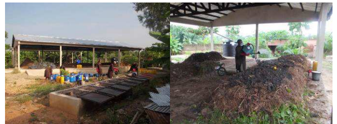
Fig. 5: Excreta hygienisation treatment (left) and co-compost windrow making process (right) (source: A. Dubois, 2014)
