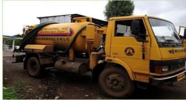
Suction emptier truck of 3KL capacity in Sinnar
