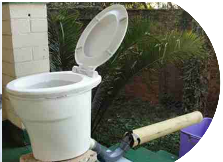
Fig.4. The MaP test was performed using up to six 50g replica stool samples and a prescribed amount of toilet paper (20 squares of single ply).
