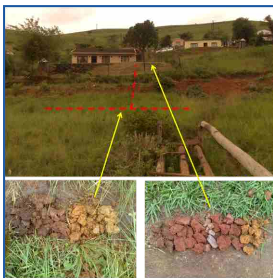
Fig.11. Location of piezometers and indication of soil types (mostly dolerite underlying geology) at the Azalea site.
