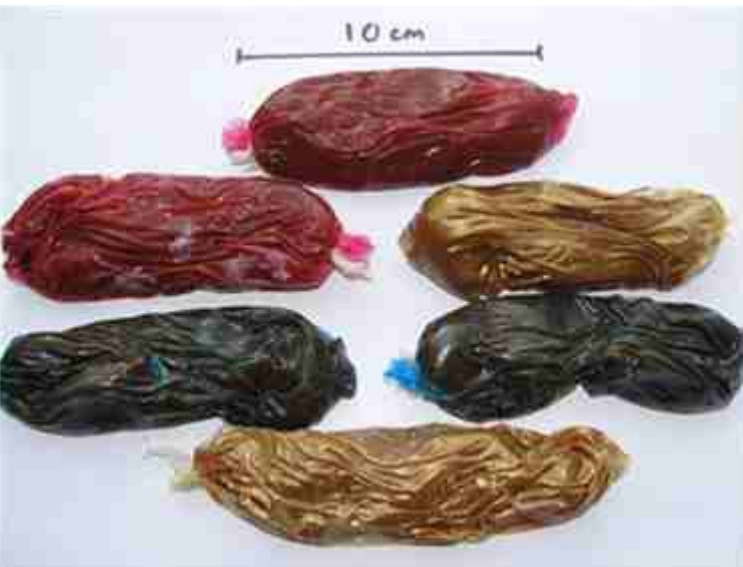
Fig.3. Replica faecal samples as described by the MaP test protocol. Each sample contains 50 grams of soy paste, and is contained in a latex sheath.
