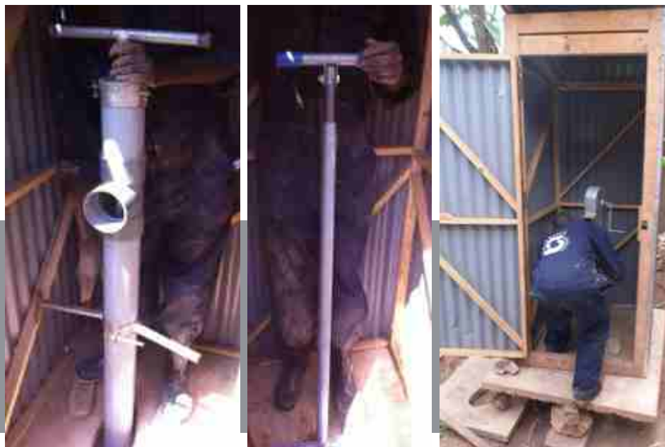
Fig.3. The research team testing each semi-mechanised device using synthetic sludge of different shear strengths. After testing, they field tested the devices with local pit emptiers to gain feedback on which technology they preferred.
