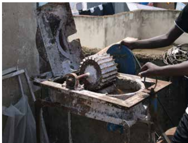
A pulping machine used to make sanitary pads from water hyacinth (Photo: Lars Marcus Vedeler)
