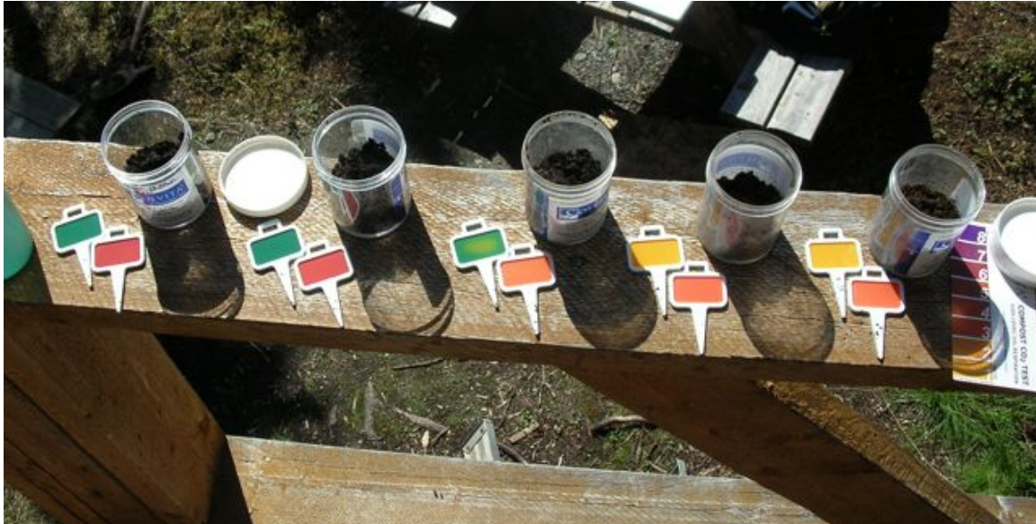
Figure 5.1. Photograph of using Solvita® compost stability and maturity tests in the field.
