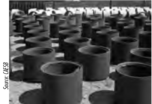
Mass production of simple concrete manholes in Brasilia
