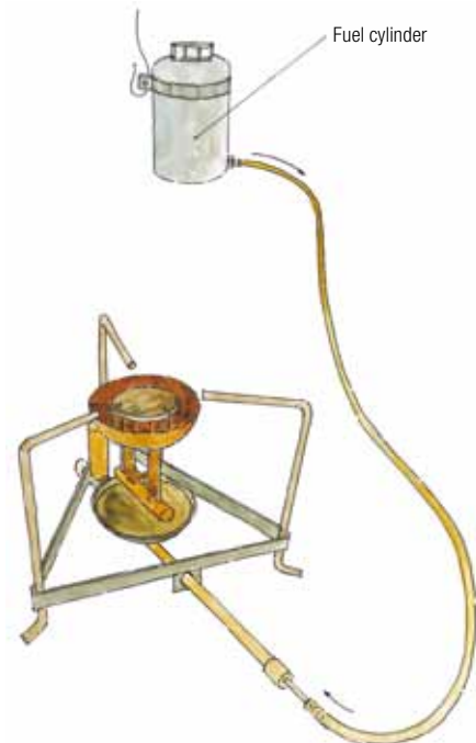
Figure 86 Gravity-fed kerosene burner
