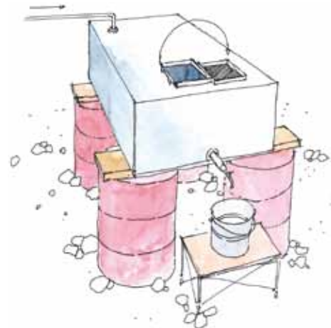
Figure 26 Improvised storage tank
