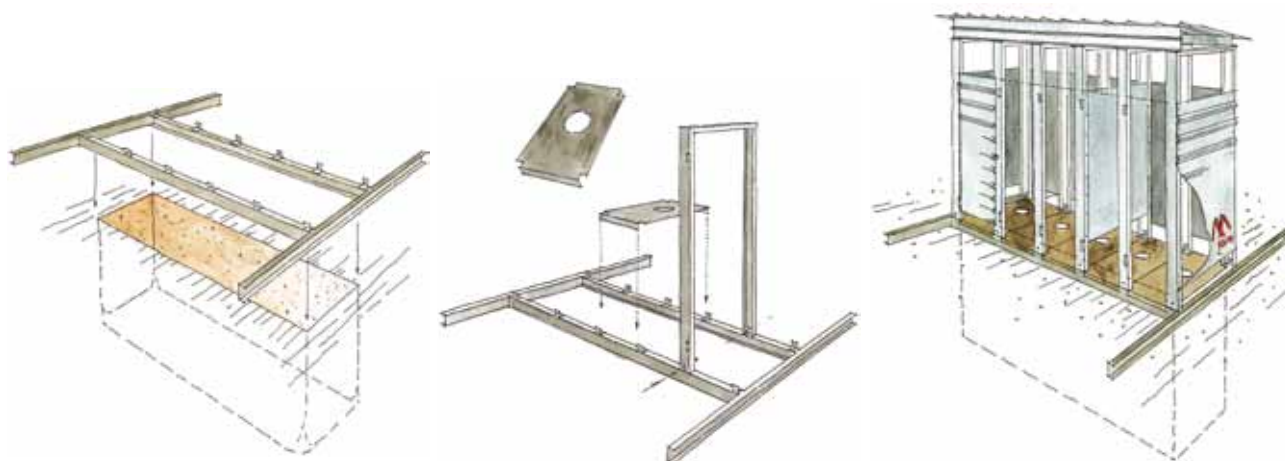
Figure 42 Block of dry pit latrines
