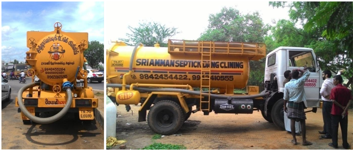
Figure 3: Vacuum tankers used for emptying onsite sanitation systems (Source: Bhitush, Rahul/CSE, 2015)
