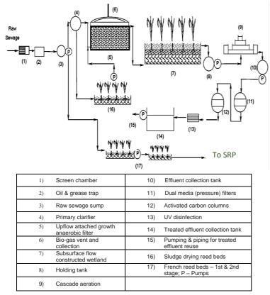
Fig. 3: Scheme of the overall treatment system (source: NEERI, 2014)
