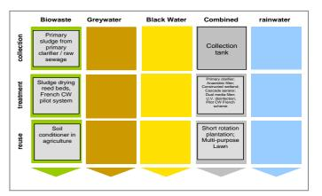
Fig. 2: Applied sanitation components in this project
