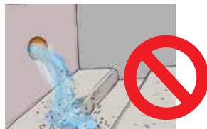
Filter media being washed out
