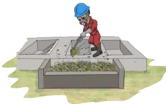
Storage of the dry waste in the solid waste chambers
