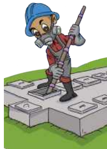
Monitoring of sludge level
