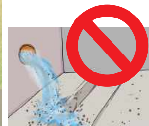
Filter media being washed out
