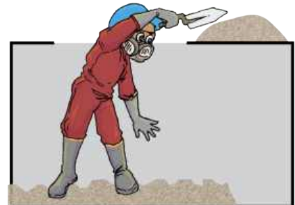
Removal of grit and settled sludge
