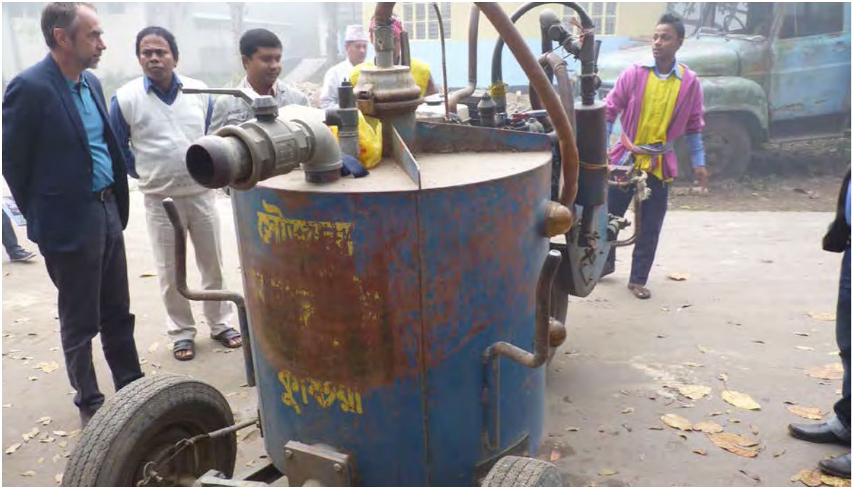
Figure 17. Vacutug, another option for narrow streets. Vacutugs are available in a variety of sizes. 0.5 to 1.6 cubic meters are most common.
