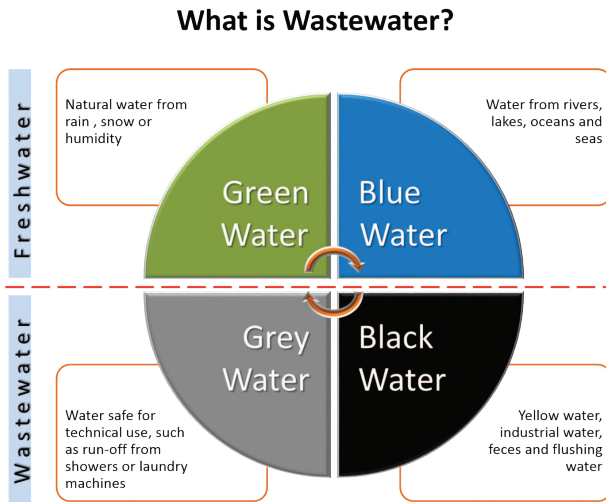
Figure 1: Basic colour code for wastewater
