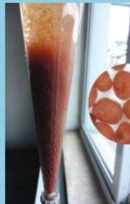
Going green. With this color, engineers gauge the density of the sludge of anammox bacteria (lower), a new way to densify wastewater.
