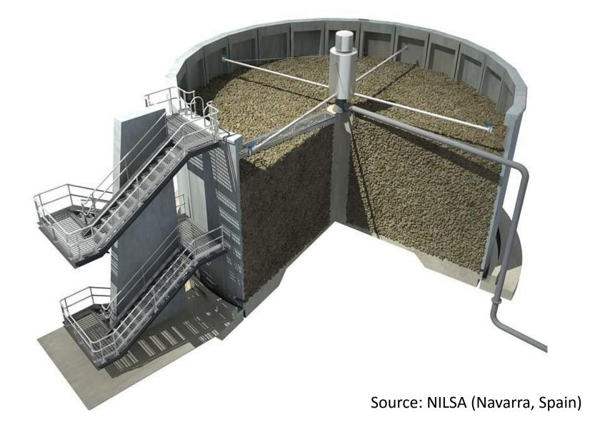
Original TF used rocks as the support media; currently, engineered plastic packing with high surface area/volume ratios with high void volumes, to avoid blockages and to achieve high loading rates.
