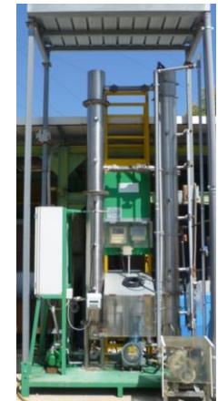
SBBGR – Innovative Compact WW treatment unit
