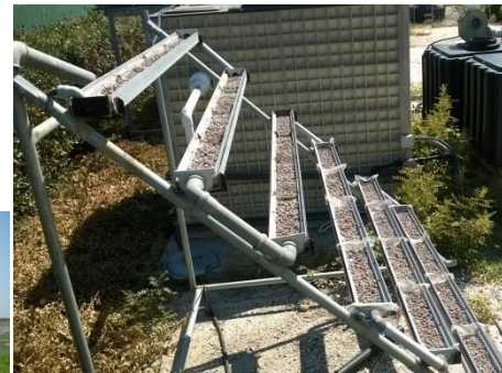
TiO 2 -coated Clay Aggregate In Novel Inactivation Unit
