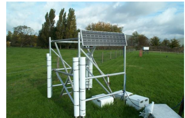
COSMOS soil moisture sensors "Area based"
