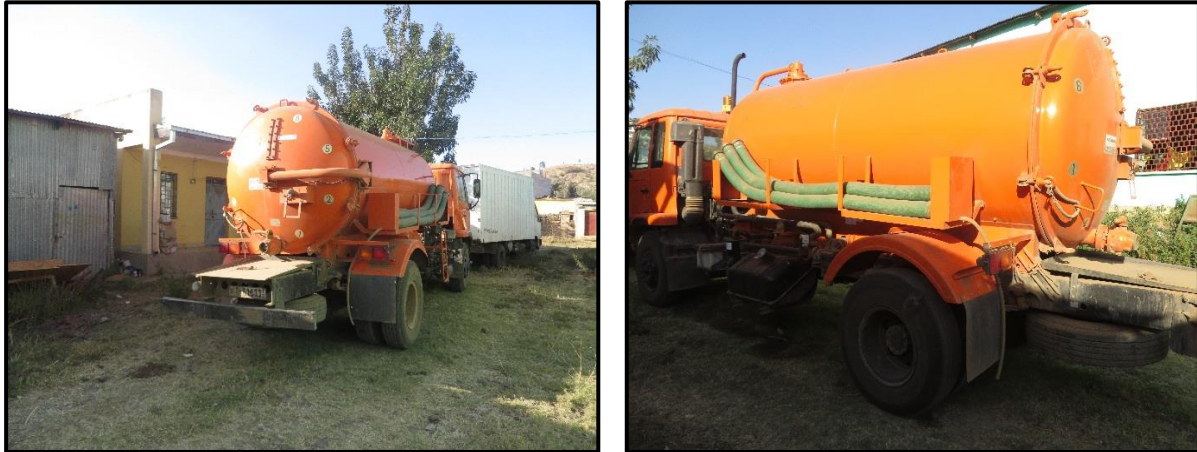
Figure 4: 8m 3 vacuum truck owned by the municipality (photo credit: Oscar Veses).
