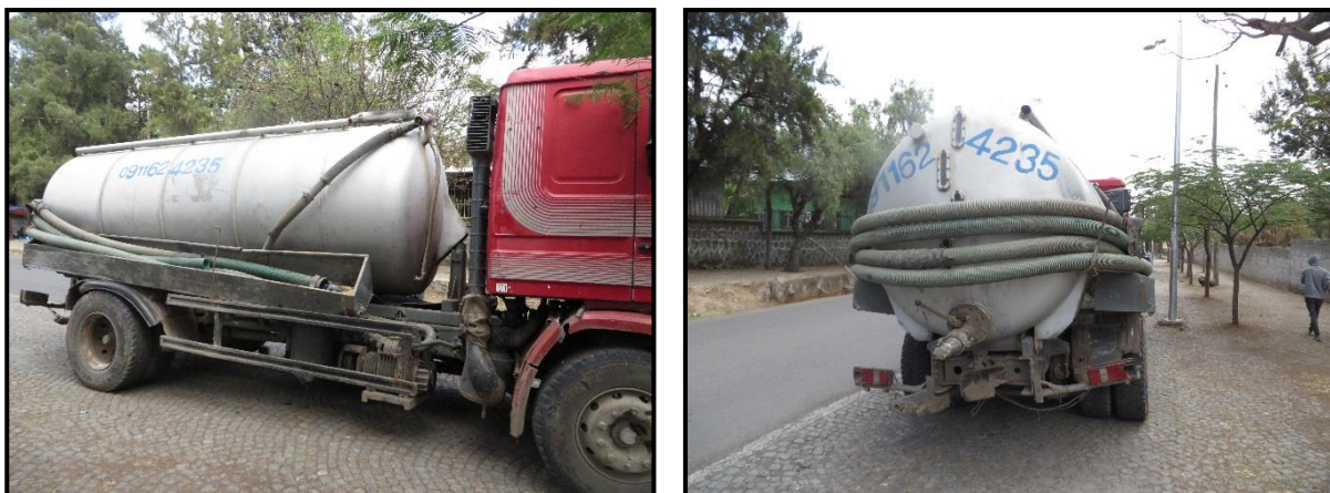
Figure 6: 10m 3 vacuum truck owned by one of the private companies (photo credit: Oscar Veses).
