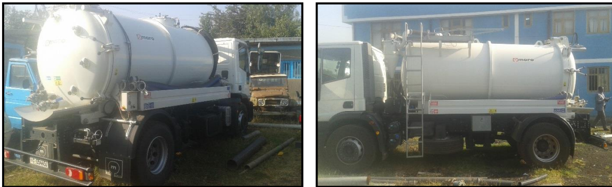
Figure 3: Two operative vacuum trucks with no current use by the BTWSSSE (photo credit: Oscar Veses).
