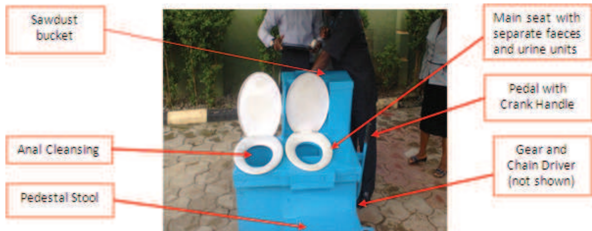
Figure 4. Features of the dry composting toilet
