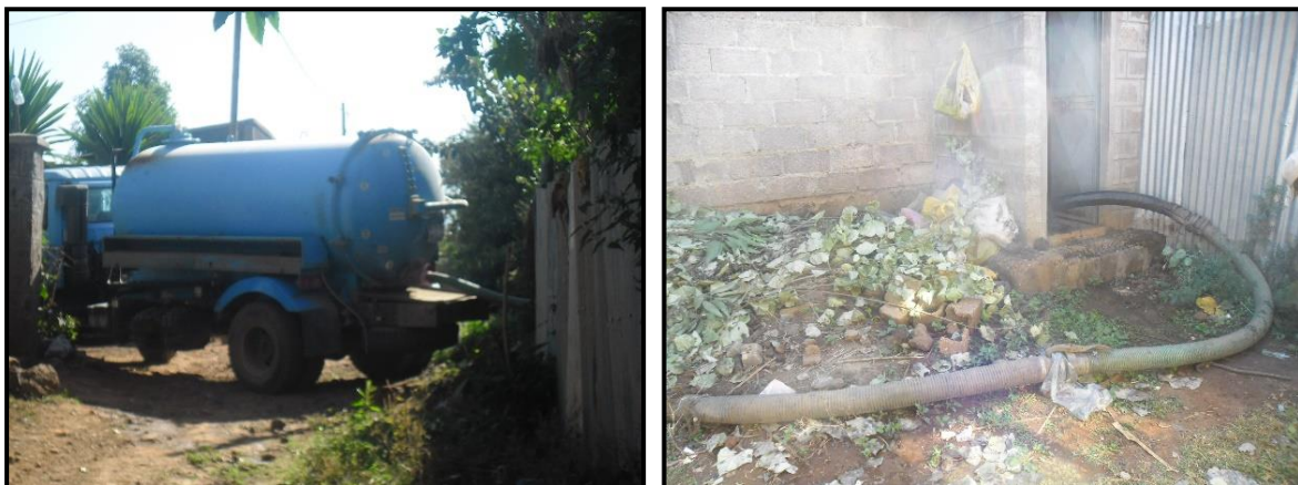
Figure 9: a) Vacuum truck owned by one of the private companies. b) Latrine emptying using a hose (photo credit: Eshetu Assefa).
